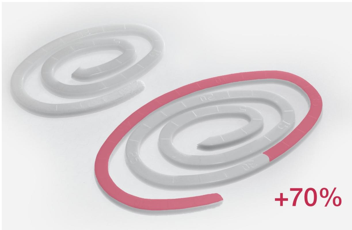
*BRUGGOLEN® TP-P1810 significantly enhances the flow of semi-aromatic polyamides such as PA6T, PA6T/6I, PA6T/6.6 while maintaining mechanical properties. © Brüggemann*
